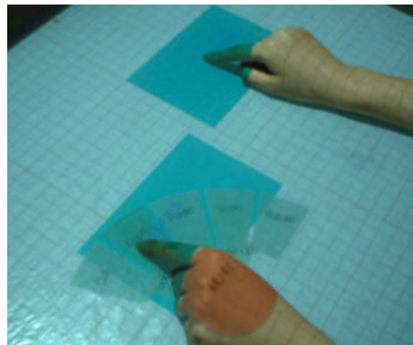
c. Left hand is used to specify the object to be copied and to select "Copy" item under "Tool" menu. Right hand specifies the position to past the object.
