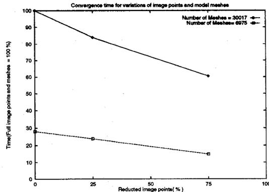
Figure 6: Convergence time for variations of image points and model meshes
