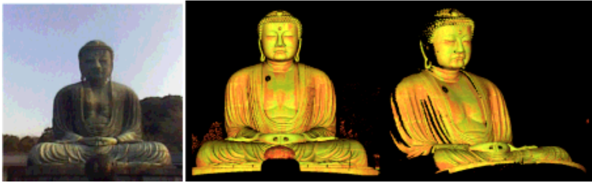
Figure 7. A color image and range image with reflectance attribute of the huge buddha in Kamakura city.
