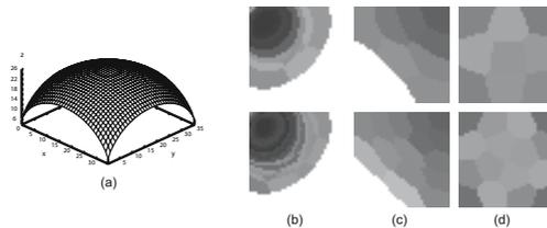
**Fig. 2.** (a) 3D shape of a target object and segmentation results of the object under (b) a point light source, (c) a set of point light sources with an area distribution, and (d) uniform illumination
