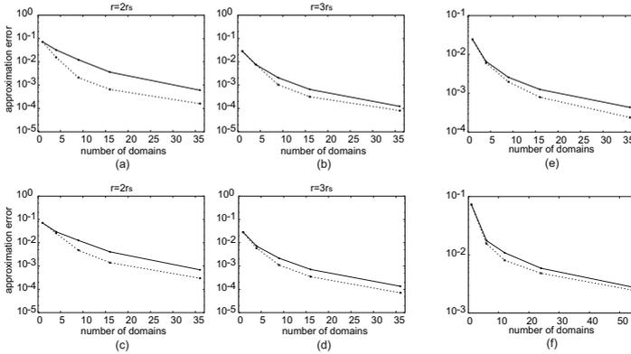
**Fig. 4.** Reconstruction errors of sphere images against the number of domains under a point light source located at (a)  $2r_s$  or (b)  $3r_s$ , and under a set of point light sources located at (c)  $2r_s$  or (d)  $3r_s$ . The solid and dotted lines represent the errors of rectangular segmentation and our method respectively. Reconstruction errors of images of a plaster sphere and those of a Napoleon figure are shown in (e) and (f).
