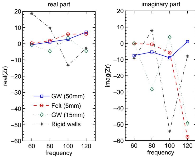
Figure 4: Complex acoustic impedance (normalized values) obtained from the experiments.
