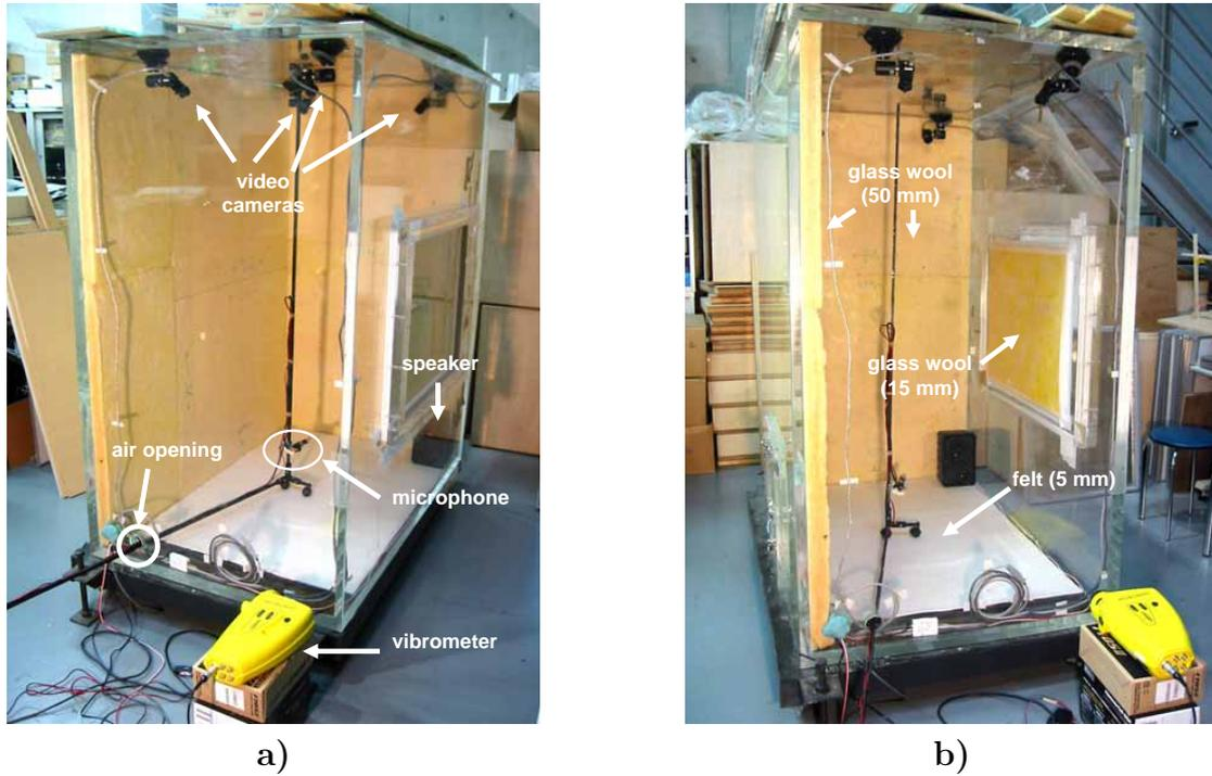
Figure 3: a) The actual experimental setup. b) Materials and surfaces considered for the preliminary experiments.
