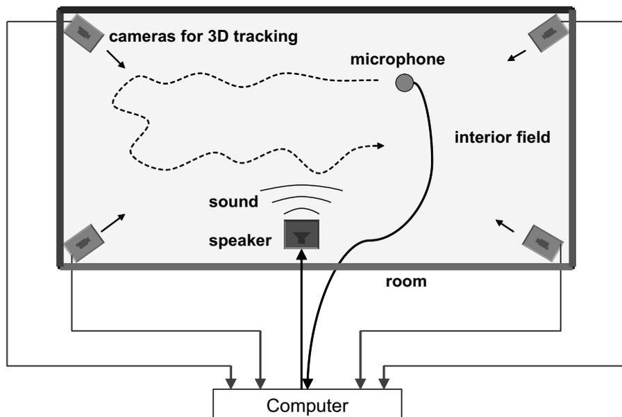
Figure 1: Setup of the inverse estimation of the acoustic impedance on the interior surfaces of a room.
