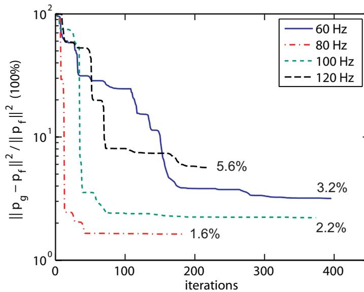
Figure 5: Convergence history of the iterations for the estimation of  $\mathbf{z}$  with the experimental data.
