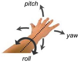
**Figure 3. Roll, pitch, yaw orientation of a hand**
