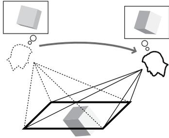
**Figure 1:** Illustration of head-coupled perspective
