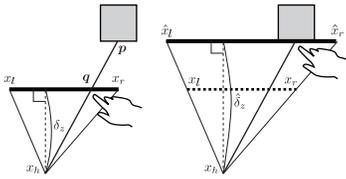
**Figure 3:** Touch-consistent perspective with adaptive relocation of the target plane
