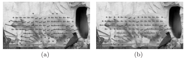
Fig. 2 The comparison of the optical flow before and after the color-guided refinement. (a) Before the refinement, there are some noises in the boundary region. (b) After the refinement, some noises are removed.
